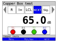
If there is no crosstalk between line pair 1 and line pair 2 (adjacent line), a maximum value is reached (in this example 65 dB).
