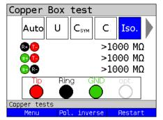
The example shows the measurement of a resistance between Tip/Ring, Tip/ Ground and Ring/Ground of > 1000 M $\Omega$ . This indicates that the line is not damaged. Depending on the requirement, a value of e.g >300 M $\Omega$  is considered good. Values <300 M $\Omega$  and >5 M $\Omega$  should be examined more closely. Values under 5 M $\Omega$  indicate an isolation fault.
