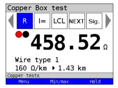
The example shows a measurement of 458  $\Omega$ . For a copper cable with a specific resistance of 160  $\Omega$  / km, this indicates a short-circuited twisted pair with a length of 1.43 km
