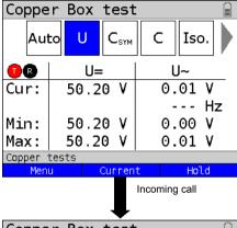
In this example the Copper Box is connected so as to measure the voltage of an POTS access.
