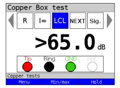
If the two wires are symmetric, i.e. identical in their mechanical properties, a max. value is measured (in this example > 65 dB). Such a high value can only be expected in ideal situations or in the event of a short circuit between Tip and Ring or an extremely short open line. A value greater than 65 dB means that the result is above the measuring range.
