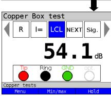
It is not possible to change the socket combination for LCL measurement.
