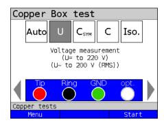
In this example, sockets Tip, Ring and GND are selected.
