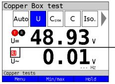
The example here shows a low-ohm (loaded) measurement.
