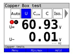
The measured voltage of 60.93 V could indicate an POTS access
