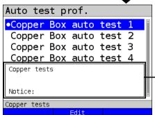
The default is the most recently used auto test profile, in this example Copper box auto test 1.
