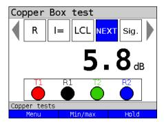
If a value <37 dB is measured, or even 5.8 dB as in this example, there may be a short between the two wire pairs. The tone is 100 % cross-coupled and severely interferes with the line.
