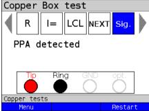
In this example, a passive test termination (PPA) was detected between Tip and Ring.
