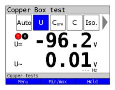
The measured DC voltage of 96.2 V can indicate an ISDN-BRI U access.
