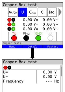
Ideally, no AC voltage should be measured between individual wires. Still, AC voltages can be coupled to the wires directly via a line termination or indirectly through the air.
