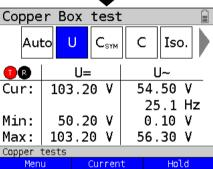
This example shows an incoming call. In addition to the DC voltage, we can see a call-switching voltage with the typical frequency of 25 Hz.
