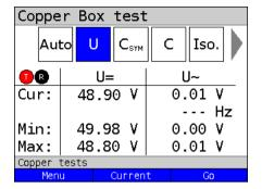
The measured DC voltage of 48.90 V can indicate the POTS access of a PBX.
