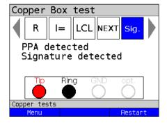
In this example, a PPA and a signature circuit between Tip and Ring were detected.
