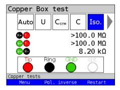
In this example, the measurement shows a markedly low resistance between Ring and Ground. This indicates a fault. Ideally, the values of Tip to Ground and Ring to Ground should always be in balance.
