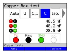
Ideally, the line should be in capacitive balance. However, if the capacitance between Tip and Ground and between Ring and Ground differ by more than 2-3 %, this can indicate an asymmetry. You can investigate this hypothesis by measuring the symmetry (see Chapter 8), which delivers a much more accurate determination of symmetry.
