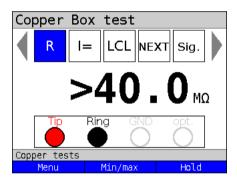
A large value such as 20 M $\Omega$  or >40 M $\Omega$  indicates that no line loop (intentional shorting) has been set up. Loop resistance cannot be measured then
